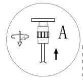
When adjusting the height of the steel wire, the telescopic metal part A toothed outer ring can only twist half a turn, and then pull it up to adjust the height!!! IMPORTANT: Test sockets with bulb before dressing the fixture.
